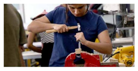
The Fitting Shop is a place where the students refine their products to achieve desired shapes, size and accuracy, through various finishing operations such as marking, filing, chipping, sawing, scraping, drilling, reaming, tapping, threading and grinding etc. The Fitting Shop includes, Machine Vice, Bench and Hand Drill Machine, Angle Grinder 540W with Angle Polisher Attachment, and various files etc.
