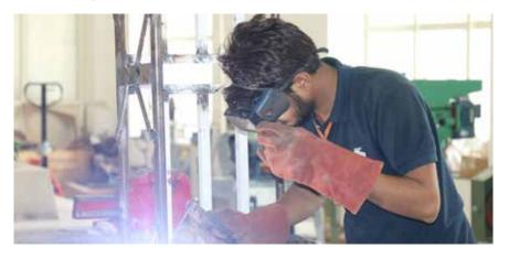
Welding Shop is a place where the students perform arc welding fusion processes for joining metals. The different operations practiced by students in Welding Shop are Position Welding, Butt Welding, Lap Welding, Spot Welding, etc. The Welding Shop includes ARC+ Tig Welding Machine with safety equipments.
